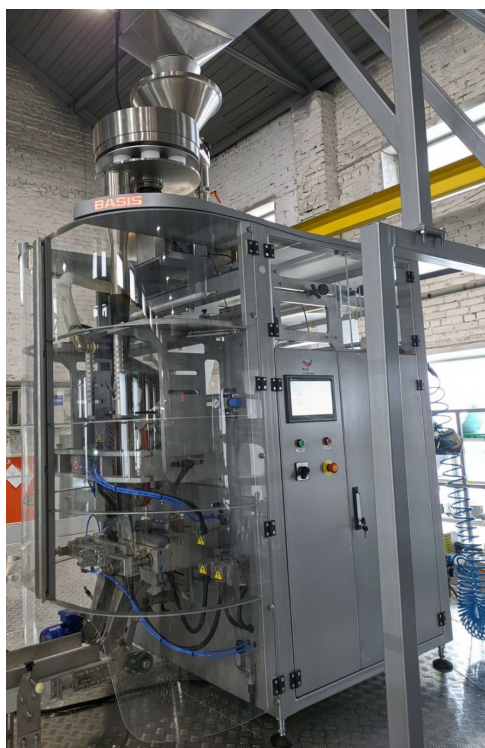
Figure 2 – Experimental installation for determining the duration of bulk products from measuring cup in a package:
